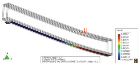
Fig. 5c Plastic damage in polymeric matrix
