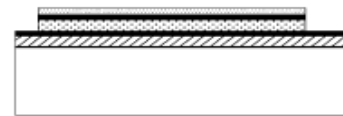
(e) Dry etching of upper electrode Pt and PZT after photo-resist patterning
