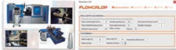
Metal-forming processes analysis: industrial equipment (left) and GUI for process parametrization (right)
