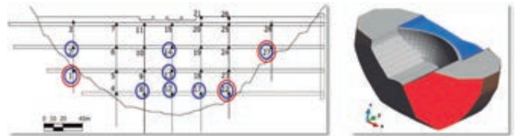
Anomaly detection in dams: example of monitoring network (left) and numerical model to simulate anomalous events (right)
